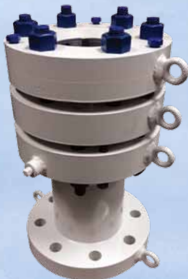
PLIDCO® Clamp+Sleeve for coupling or repairing badly damaged pipe. Packing assures a positive seal and clamping surfaces grip the outside pipe wall to counteract end-pull and axial stresses.
