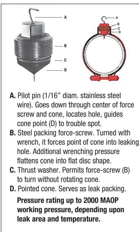
**A.** Pilot pin (1/16" diam. stainless steel wire). Goes down through center of force screw and cone, locates hole, guides cone point (D) to trouble spot.
