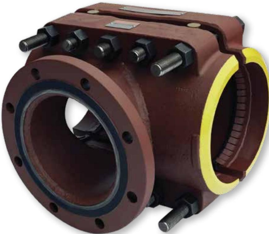
PLIDCO® Hot Tapping+Saddles are designed to ASME code section VIII and meets the intent of API 6H/6X to make *branch connections* on existing pipelines or for *plugging* operations without welding. They are easily installed by simply tightening the side bolts. Steel GirderRings hold seals in place to protect from damage and displacement during installation. When conditions are favorable, PLIDCO® Hot Tapping+Saddles can be permanently welded to the pipeline.
